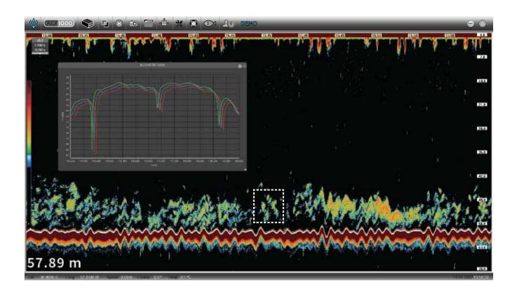
All objects detected by an echo sounder present different sound responses, depending on its shape and density. The frequencies contained in a sound pulse are also key to determine the way an object will respond to sound. That is how certain species of fish respond with a higher intensity than others to a certain frequency.
